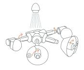
To remove the **Pressing units** for in-depth cleaning of their parts, turn the **Fasteners** of the pressing units a quarter of a turn.
