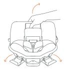
Open the fasteners to remove the **Cover** for cleaning, pulling upwards as indicated in the drawing, taking care with the flanges.
