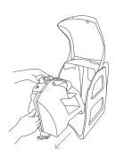
Pull the **Juice extraction unit** out, sliding it along the guides until it is fully released.
